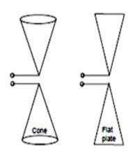
Fig 2: Few wideband Bowtie antenna types
