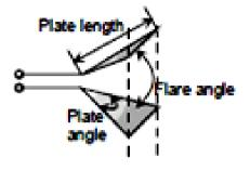
Fig 3: Folded horn antenna
